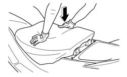
(2) Install the rear seat. Make sure that the seats are securely installed before operating the watercraft.
