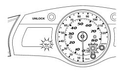
If this occurs, reduce the engine speed, return to shore, and then check the engine oil level. (See page 61 for engine oil level checking procedures.) If the oil level is low, add enough engine oil to raise it to the proper level. If the oil level is sufficient, have a Yamaha dealer check the watercraft.
