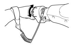
(3) Check that the angle of the jet thrust nozzle changes when the QSTS selector is shifted from neutral to bow up or bow down.
