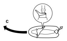
D. If the engine is stopped while riding, there is no thrust. The watercraft will go straight even though the handlebars are turned.
