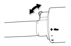
(2) Check that the QSTS selector turns smoothly when the lever is squeezed and check that the selector locks in place at each position when the lever is released.
