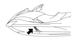
To check for proper operation of the cooling system, check that water is being discharged from the port (left) pilot outlets. If water is not being discharged from these outlets, cooling water may not be circulating in the engine. When this occurs, stop the engine and check
