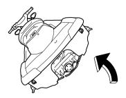
(2) Remove any weeds or debris from around the jet intake, drive shaft, impeller, jet pump housing, and jet thrust nozzle.
