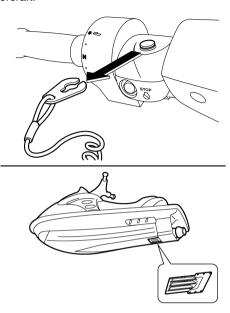
(1) Place a suitable clean cloth or carpeting underneath the watercraft to protect it from abrasions and scratches. Turn the watercraft on its side as shown. NOTICE: Always turn the watercraft over onto its port (left) side. When turning the watercraft on its side, support the bow so that the handlebars are not bent or damaged. [ECJ00661]
