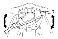
Push the handlebars back and forth to check that the tilt lever and handlebars are locked in place. (See "Tilt lever" on page 35 for more information.)
