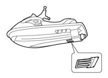
Engine shut-off cord (lanyard)
