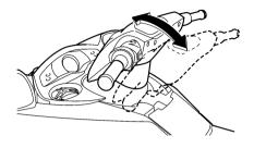
Make sure that the tilt lever returns to its original position and that the handlebars are locked in place after adjusting them.
